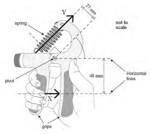
The diagram shows the gripper being squeezed. In this situation, the gripper is in equilibrium. The force produced by the fingers is equivalent to the single force  $\boldsymbol{X}$  of magnitude 250 N acting in the direction shown above. A force,  $\boldsymbol{Y}$ , is exerted by the spring which obeys Hooke's law.
